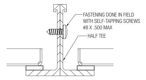
Figure 16: Fastened Adjacent Ceiling Sections
