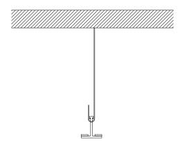
Figure 11: Temporary Hanger Wire Support
