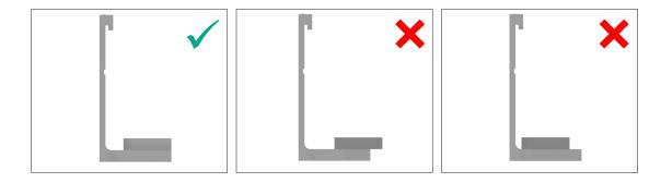
Figure 9: Gasket Installation Cross Section
