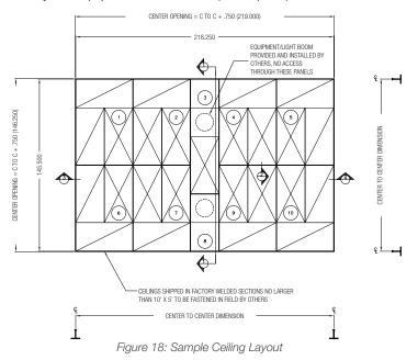
Step 16: Identify ceiling panel locations, denoted with a letter on the job specific submittal. There are three types of ceiling clips used on the HGWC systems.
