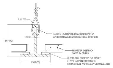
Figure 15: Perimeter Installation Detail
