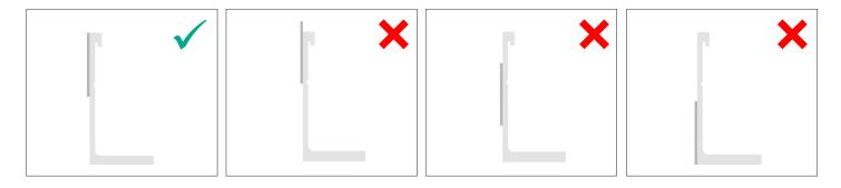
Figure 10: Half Tee Field Joint
