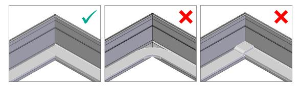
Figure 8: Gasket Installation Isometric View
